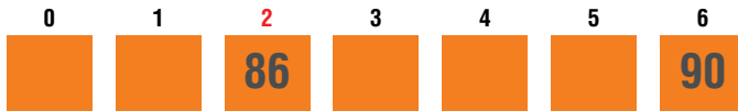
Figure 13.3: To store 90 in the hash table, you perform modulo by the number of slots and get 6.
