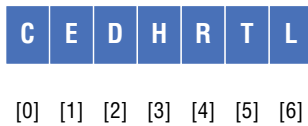
Figure 15.12: An array with keys at indexes based on their position in the tree.
