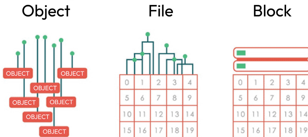
Figure 2.1 – Object storage, filesystem, and block storage
