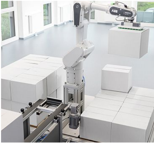
With a higher reach and payload capacity than other collaborative robots, the SWIFTI CRB 1300 is 44% faster than other cobots, said ABB. Credit: ABB
