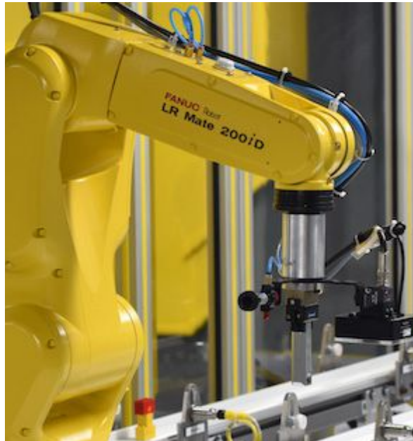
FANUC's LR Mate 200iD/7C clean room robot is resistant to water and dust in accordance with IP67.
