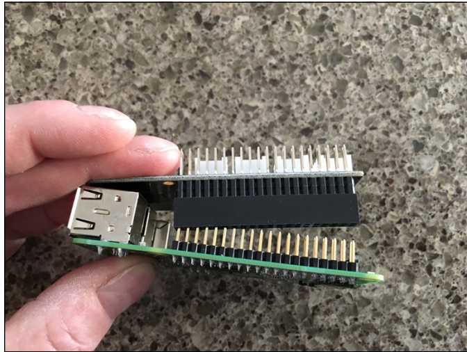
FIGURE 1-5: Aligning the Pi2Grover board with the Raspberry Pi.
