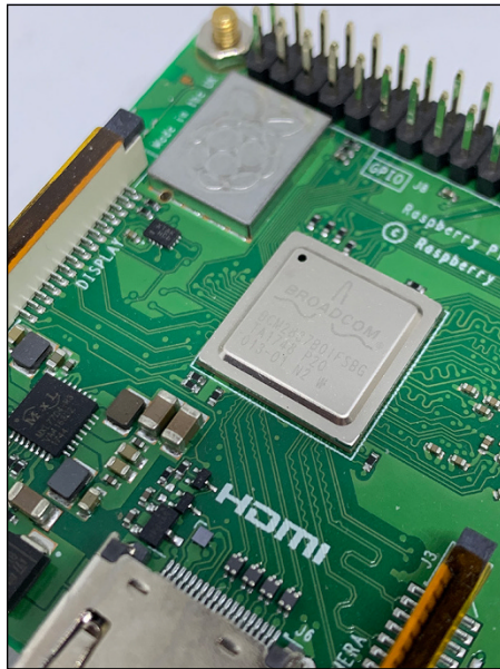
FIGURE 4-1: The Raspberry Pi 3B+ processing chip containing the Videocore-IV.
