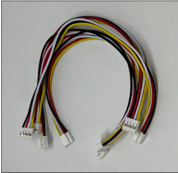
FIGURE 2-10: 20cm Grove cables.
