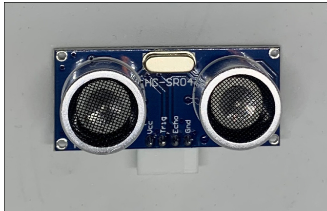
FIGURE 2-8: An ultrasonic distance sensor.
