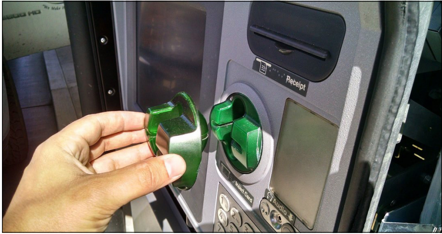
FIGURE 5-5: A card skimmer on an ATM.
