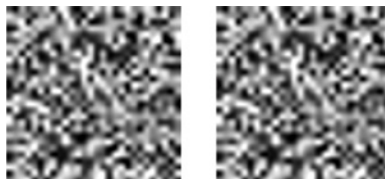
Figure 3.7 The attacker can start with any image and modify it to something the ML system recognizes. The image on the left is recognized as a 1. The image on the right is recognized as a 6.
