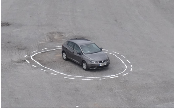
Figure 2-8 A self-driving car is immobilized because it confuses the salt circle for lane markings.
