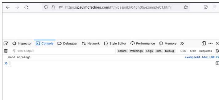
FIGURE 5-1: An example of calling a function when the <script> tag is parsed.
