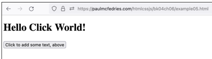
FIGURE 6-6: The click event callback function adds some HTML and text to the div element.
