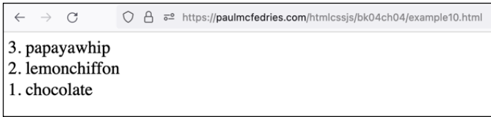
FIGURE 4-3: The decrementing value of the rank variable is used to create a reverse-ordered list.
