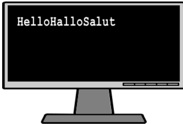
Figure 6–2 The output result displays on one line. In order to output a “line break” you must put the special sequence of characters \n after every word.
