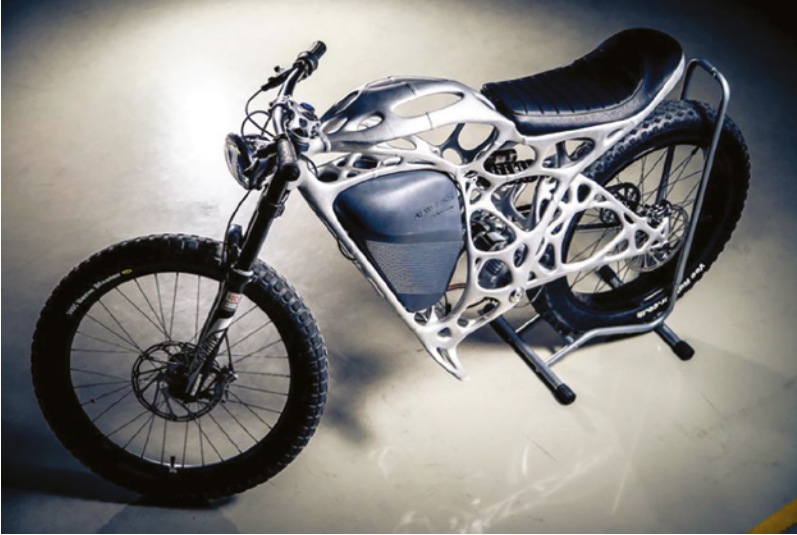
FIGURE 3.5 Airbus APWorks launches the Light Rider, the world's first 3D-printed motorcycle.
