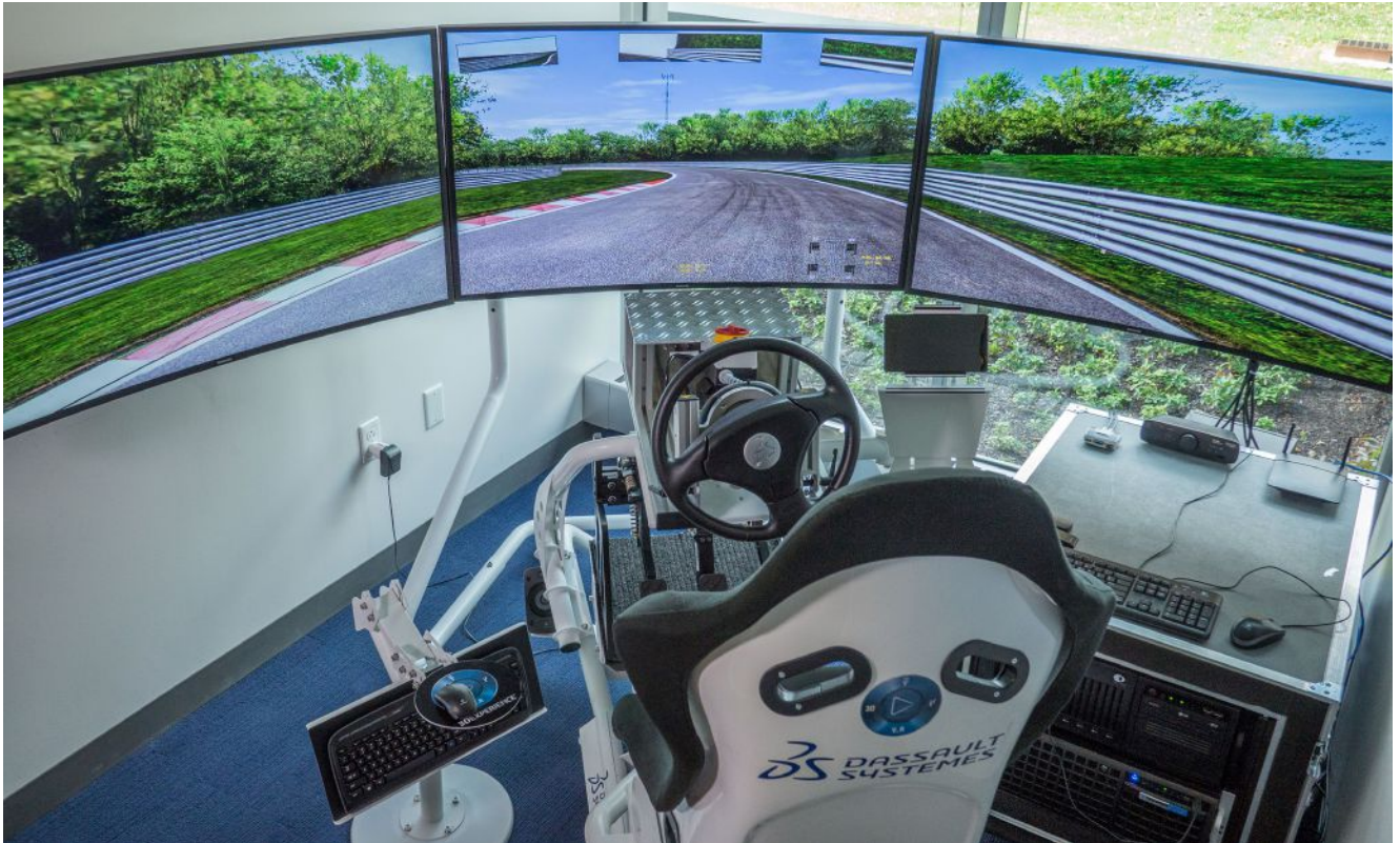
SIMULIA Simpack driving simulator enables product development teams to experience real-time vehicle performance in a range of operating conditions by integrating software-, hardware- and driver- in-the-loop capabilities. Image courtesy of Dassault Systèmes.
