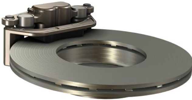
CAD model of a brake assembly. Image courtesy of COMSOL.
