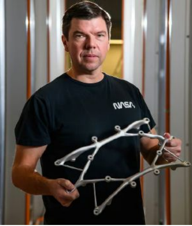
NASA uses GD software for a variety of applications. NASA Research Engineer Ryan McClelland shows a structural mount designed using GD, and 3D printed in titanium. Image courtesy of NASA.
