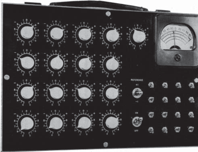
Figure 2.6 Photograph of the Adaline developed at the Stanford Electronics Laboratory at the University of Stanford in 1960. This is possibly the first electronic learning device to use a gradient descent approach. Source: Widrow and Hoff (1960).
