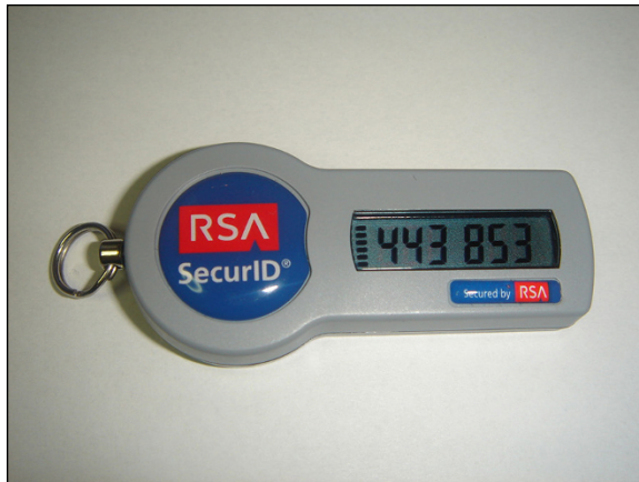
FIGURE 8-4: An RSA SecurID brand one-time password generator hardware token.
