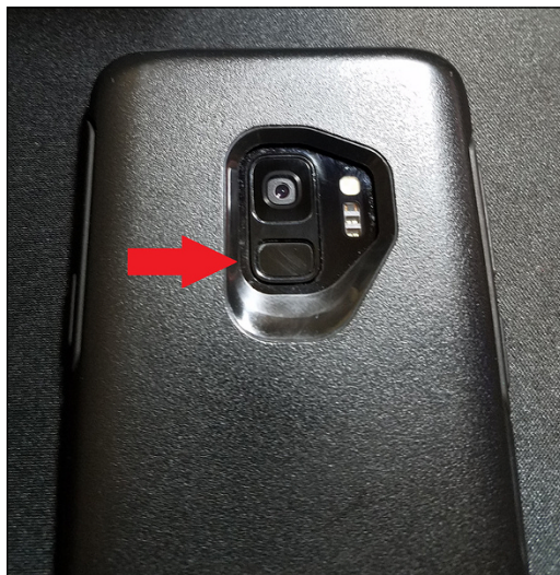
FIGURE 8-3: A phone fingerprint sensor on a Samsung Galaxy S9 in an Otterbox case. Some phones have the reader on the front, while others, like the S9, have it on the back.
