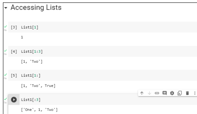
FIGURE 13-2: Knowing the correct indexing operation to perform is important.
