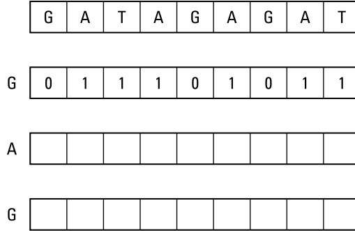
FIGURE 3-4: The Shift Or algorithm creates an array of matching characters.
