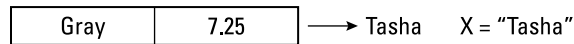
FIGURE 4-7: The Peek command retrieves data, but the Dequeue command retrieves and removes data.
