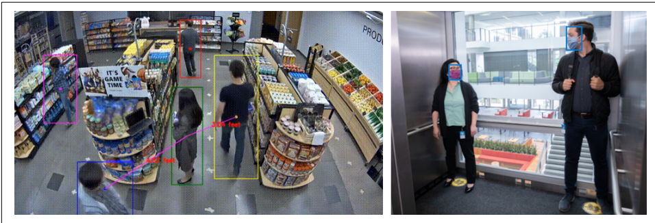
Figure 14-5. Using spatial analysis to verify social distancing and masking (images © Microsoft; used with permission)
